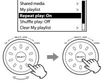
Each time the SELECT button pressed, the repeat or shuffle mode changes on and off.
